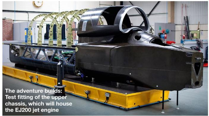
The adventure builds: Test fitting of the upper chassis, which will house the EJ200 jet engine
