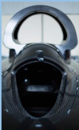
Sandwiched between the layers of carbon fibre are three thicknesses of aluminium honeycomb core – 8mm, 12mm and 20mm – which provide additional strength. At its thickest point the monocoque comprises 13 individual layers, but is just 25mm in cross-section. The structure weighs 200kg and bolts directly to the metallic rear chassis carrying the jet, rocket and racing car engine.
