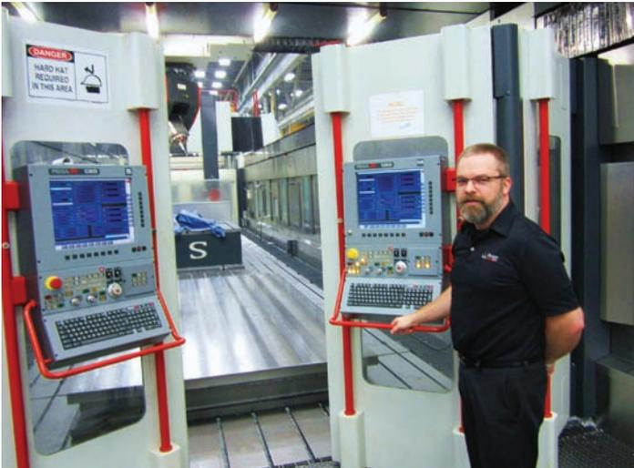
Brian Kerkstra, Paragon Die & Engineering Manufacturing Engineer, shows Fidia's 60 ft. long Y2G twin spindle gantry 5-axis CNC milling machine, one of the four Fidia machines that Paragon has. There are dual controls at each end of the machine so it can be operated from each end.
