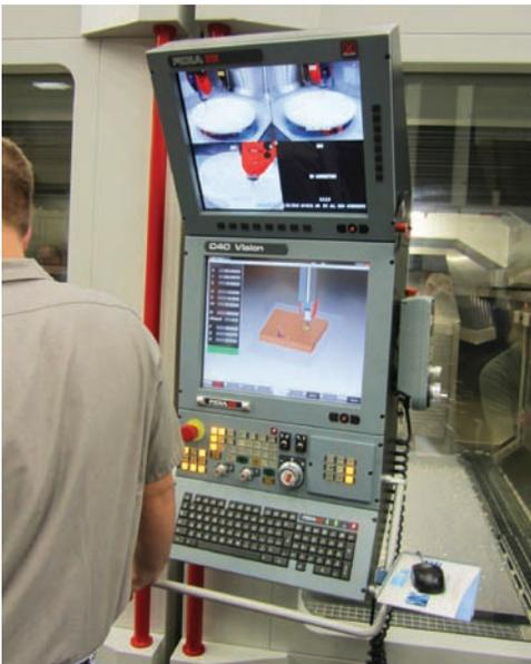
Fidia's new flagship C40 control has a dual screen with ViMill Look Ahead virtual milling software and a four camera system to see inside the machining area when the doors are closed.
