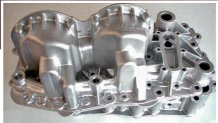
*Type of piece for the automotive sector obtained by die-casting process using Flavio Gilardoni's molds*
