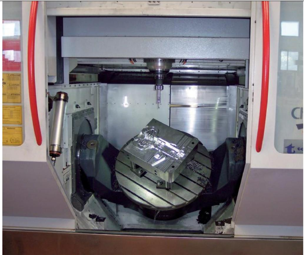
*5-axis machining on a CNC machining centre.*
