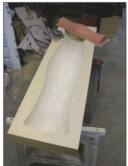
Mould used to cast the corkscrew handles.
