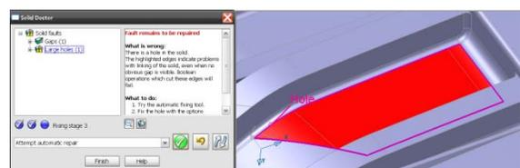
The surfaces are deleted from the solid, leaving a large hole.
