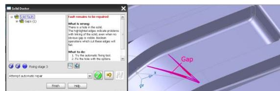
The final inconsistency is caused by a degenerate surface (possibly as a result of a translation error).
