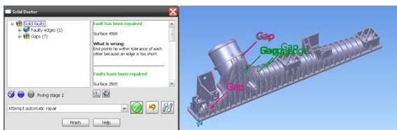
After automatic repair, issues that have been attended to are clearly highlighted, both in the graphics window and the tree, for ease of identification.
