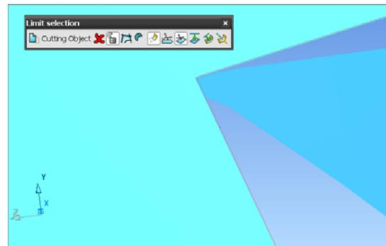
This inconsistency is repaired by re-trimming the overlapping surface to its neighbour. The two surfaces are 'sewn' back into the Parasolid model.
