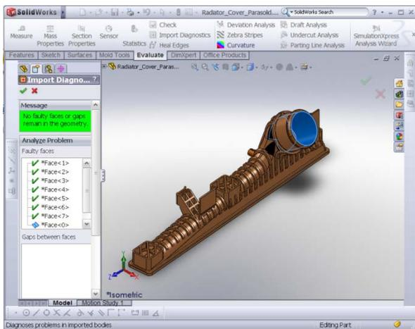
As a final test, the model was saved in Parasolid's XT file format and then imported into SolidWorks. SolidWorks' own 'Import Diagnostics' checking reported it was a valid model and further work on the design could continue immediately.
